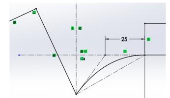
Create the **style spline** shown to complete the head of the wrench.
