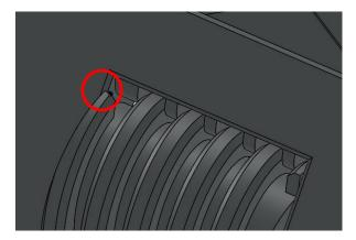
Mate this vertex to the outer surface of the cylindrical rack. Thereby, the screw thread will stop once it meets the outer cylindrical surface.
