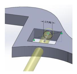
**Extrude cut** in direction 1 - **5mm** and direction 2 **Through All**.
