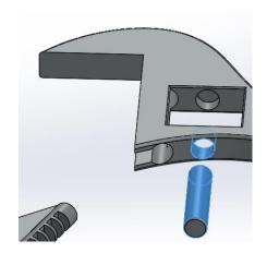
Coincident Mate between end of dowel and top of the hole.
