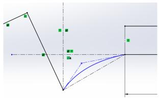
Add a **horizontal** property to the **inference line** of the spline and dimension the vertex as shown.
