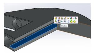
Complete the slot for the wrench jaw by creating a sketch on the inner surface.
