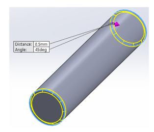
Add a **0.5mm** chamfer to either end of the dowel.
