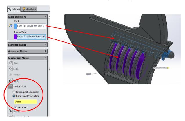
**Note:** The screw thread can now be turned to adjust the wrench jaws.
