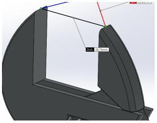
Use the **Measure Tool** to measure the distance between the wrench jaws in the fully open position.
