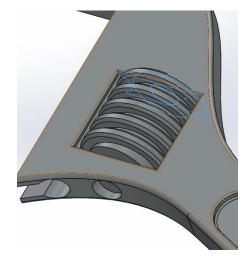
Coincident mate to place worm screw in position.
