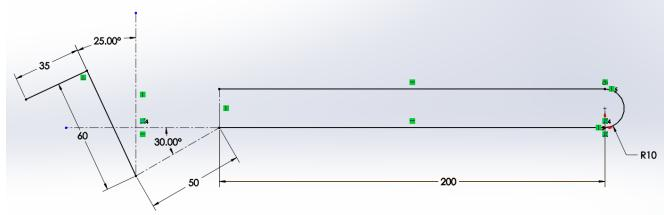
Select **Style Spline** sketch tool and draw the style Spline shown using 3 points.
