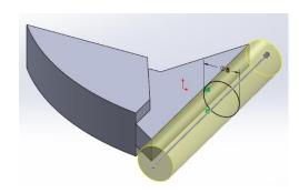
Sketch the thread cut onto the **Right Plane**
