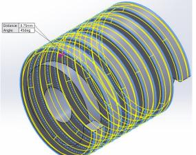
**Trim** off the excess thread on either end of the worm screw.
